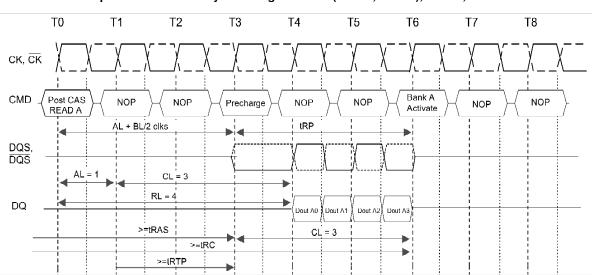
Burst Read Operation Followed by Precharge : RL = 4 (AL = 1, CL = 3), BL = 4, t<sub>RTP</sub> <= 2clocks
