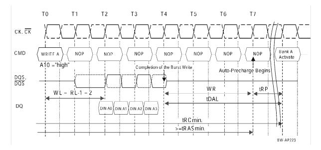
Burst Write with Auto-Precharge (t<sub>RC</sub> Limit) : WL = 2, t<sub>DAL</sub> = 6 (WR = 3, t<sub>RP</sub> = 3), BL = 4
