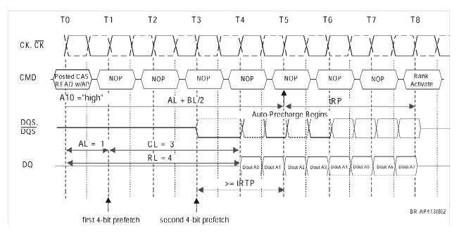
Burst Read with Auto-Precharge followed by an Activation to the Same Bank: RL = 4 (AL = 1, CL = 3), BL = 4,  $t_{RTP} > 2clocks$
