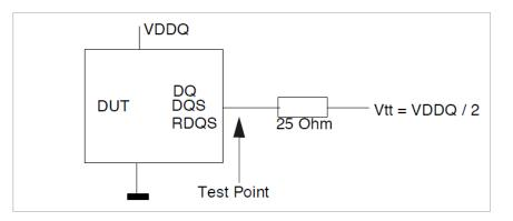
Output slew rate for falling and rising edges is measured between  $V_{TT}$  - 250 mV and  $V_{TT}$  + 250 mV for single ended signals. For differential signals (e.g. DQS -  $\overline{DQS}$ ) output slew rate is measured between DQS -  $\overline{DQS}$  = - 500 mV and DQS -  $\overline{DQS}$  = + 500 mV. Output slew rate is guaranteed by design, but is not necessarily tested on each device.
