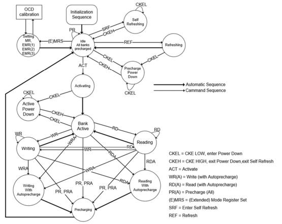
Note: Use caution with this diagram. It is intended to provide a floorplan of the possible state transitions and the commands to control them, not all details. In particular situations involving more than one bank, enabling/disabling on-die termination, Power Down entry/exit – among other things – are not captured in full detail.
