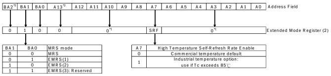
\*1: BA1 must be programmed to 0 setting the mode register during initialization.
