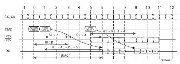
Read followed by a write to the same bank, Activate to Read delay <  $t_{RCD(min)}$ : AL = 2 and CL = 3, RL = (AL + CL) = 5, WL = (RL - 1) = 4, BL = 4
