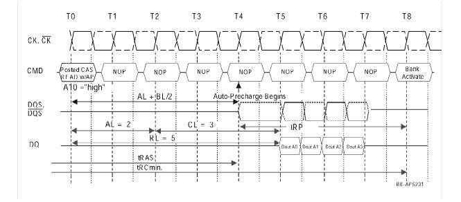
Burst Read with Auto-Precharge followed by an activation to the Same Bank ( $t_{RAS}$  Limit) RL = 5 (AL = 2, CL = 3), BL = 4,  $t_{RTP}$  <= 2 clocks
