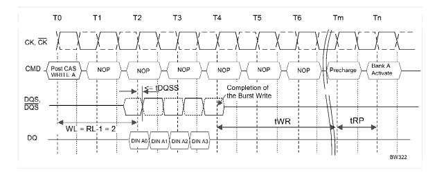
The minimum number of clocks from the burst write command to the burst read command is (CL - 1) +BL/2 + tw\_{TR}
