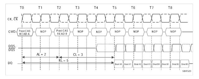
The seamless burst read operation is supported by enabling a read command at every BL / 2 number of clocks. This operation is allowed regardless of same of different banks as long as the banks are activated.
