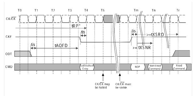
\* = Device must be in the "All banks idle" state to entering Self Refresh mode. ODT must be turned off prior to entering Self Refresh mode.
