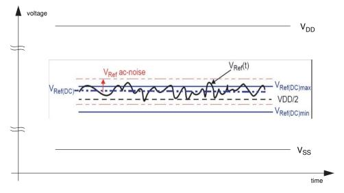
$V_{\text{REF}}(DC)$  tolerance and  $V_{\text{REF}}$  AC-Noise limits
