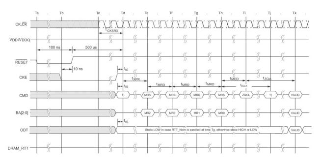
1) From time point 'Td' until 'Tk', NOP or DES commands must be applied between MRS and ZQCL commands
