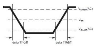
**Differential Output Slew Rate definition**
