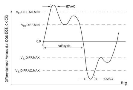
Definition of differential ac-swing and "time above ac level" t<sub>DVAC</sub>
