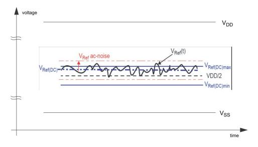
$V_{\text{REF}}(\text{DC})$  tolerance and  $V_{\text{REF}}$  AC-Noise limits
