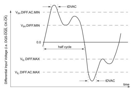
Definition of differential ac-swing and "time above ac level"  $t_{\text{DVAC}}$
