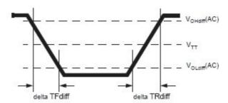
**Differential Output Slew Rate definition**
