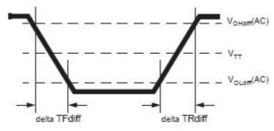
**Differential Output Slew Rate definition**
