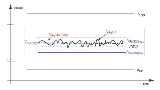
$V_{\text{REF}}(DC)$  tolerance and  $V_{\text{REF}}$  AC-Noise limits
