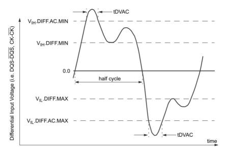
Definition of differential ac-swing and "time above ac level"  $t_{\text{DVAC}}$
