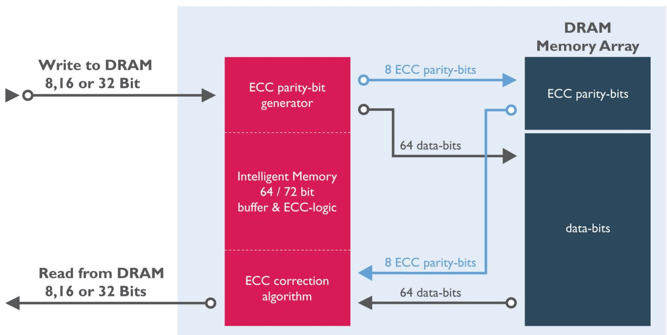
I'M ECC –DRAM with integrated error correcting code
