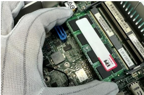
Figure 9: Insert the module into the socket at an angle
