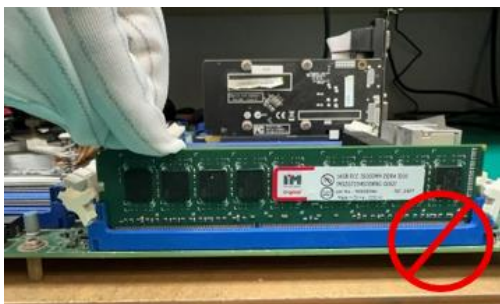
Figure 14: Do not insert a module by pushing on one side only
